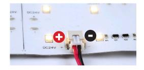
Red wiring should always be aligned to the positive charge. Black wiring should always be aligned to the negative charge.
