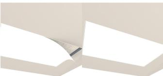
After mudding has dried, install the fabric textile into the inside edges of the frame.
