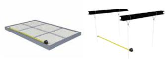
Measure positions of the suspension supports.
