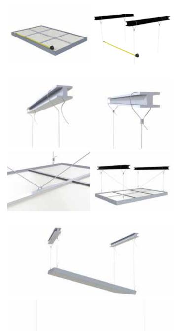
Measure positions of the suspension supports.
