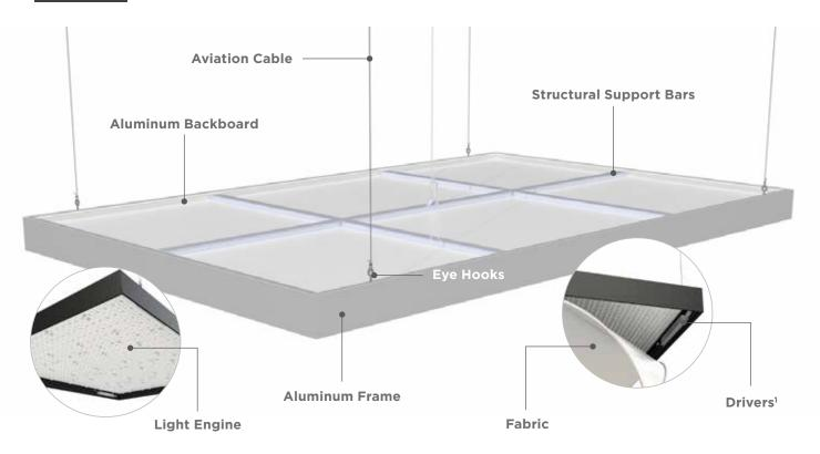
1 LUXCANVAS with remote power supplies will not contain integrated drivers inside the luminaire. For remote power supplies the driver will be mounted in a suitable location remotely from the luminaire.
