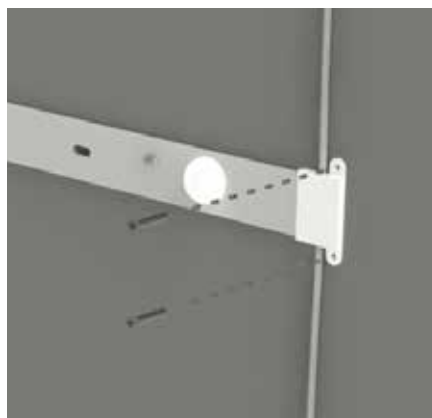
5) Use screws to fasten end caps to your substrate.
