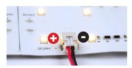
Red wiring should always be aligned to the positive charge. Black wiring should always be aligned to the negative charge.
